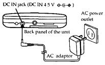
When recharging is complete, unplug the AC adaptor from the power outlet and the DC IN jack
